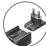
3. To remove the plug, press the tab and slide the plug away from the cable.
