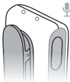
Press the button for 2 seconds until the status indicator is off.
