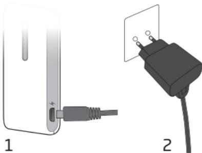
1. Insert the micro USB into the charging socket on EduMic.
