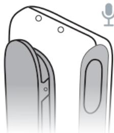
Press and hold down the button for 10 seconds until the status indicator turns MAGENTA.
