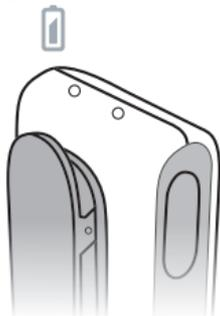
The power indicator will turn **GREEN** when the battery is fully charged.
