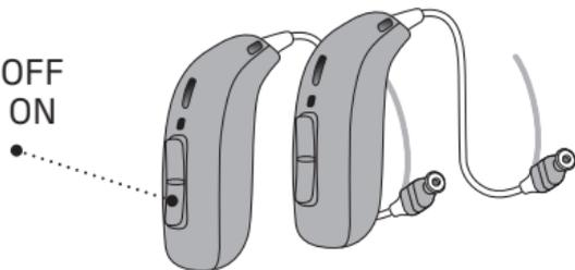
1. Turn the hearing aids OFF by pressing the lower part of the hearing aid push button for 3 seconds.
