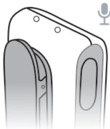
When the FM receiver is connected, the status indicator is YELLOW.
